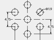
2) Suitable only for bulkhead mounted housings: HR23-BK-D2.7, HR23-BK/R-OD2.7 and HR23-BK/R-OM2.5
